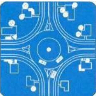
**Description:** Roundabouts require traffic to circulate counterclockwise around a center island. Unlike Traffic Circles, roundabouts are used on higher volume streets to allocate right-of-way between competing movements.
