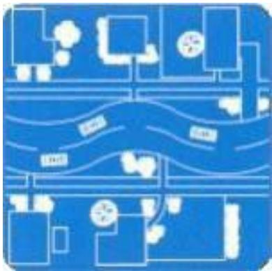
**Description:** Chicanes are curb extensions that alternate from one side of the street to the other, forming S-shaped curves. Chicanes can also be created by alternating on-street parking, either diagonal or parallel, between one side of the street and the other. Each parking bay can be created either by restriping the roadway or by installing raised, landscaped islands at the ends of each parking bay.
