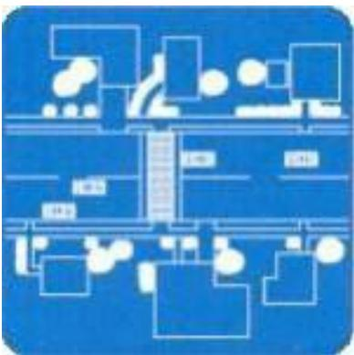
**Description:** Raised crosswalks are Speed Tables outfitted with crosswalk markings and signage to channelize pedestrian crossings, providing pedestrians with a level street crossing. Also, by raising the level of the crossing, pedestrians are more visible to approaching motorists
