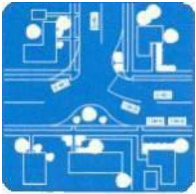
**Description:** Realigned intersections are changes in alignment that convert T-intersections with straight approaches into curving streets that meet at right-angles. A former "straight-through" movement along the top of the T becomes a turning movement. While not commonly used, they are one of the few traffic calming measures for T-intersections, because the straight top of the T makes deflection difficult to achieve, as needed for Traffic Circles.
