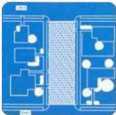
Description: Textured and colored pavement includes the use of stamped pavement or alternate paving materials to create an uneven surface for vehicles to traverse. They may be used to emphasize either an entire intersection or a pedestrian crossing and are sometimes used along entire street blocks.
